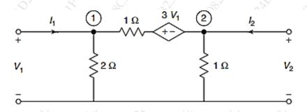
4. (A) Find Z, Y, h and ABCD parameters of given two port network shown. (10)
