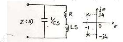
(B) Find Z and Y parameters of given two port network shown. (10
