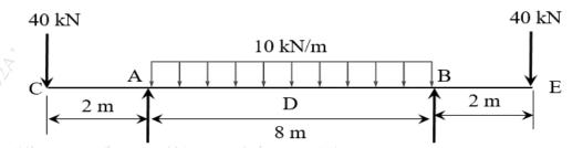
Q3 (a) Beam, A-E is loaded as shown in figure. Determine the shear force and bending (10) moment diagram.
