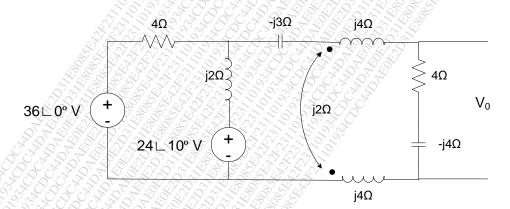
Q6 Find  $h_{12}$ ,  $Z_{12}$ ,  $Y_{12}$  and  $h_{22}$  for the given two port network . 10
