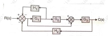
b. Obtain the transfer function for the following figure using Mason's gain formula
