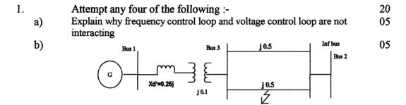
For the system shown if fault occurs at the middle of the line. Find transfer reactance between bus 1 and 2 by **NODE ELIMINATION** technique only
