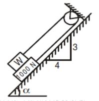
b) Determine the resultant of the given force system as shown in fig.
