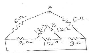
Q5 (a) Find the current through  $6\Omega$  resistance using Nodal analysis.
