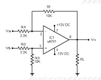
Q6.c Identify the circuit diagram. Calculate I<sub>L</sub> for this circuit.
