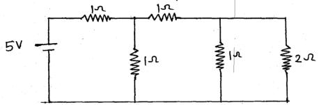
Q3 b) Find the current ly using Superposition 10
