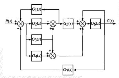
B) Find overall transfer function C(s)/R(s) for the given signal-flow graph using mason's **10 Marks** gain formula.
